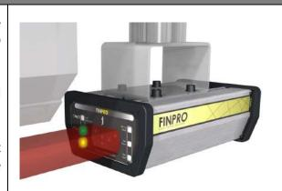
When BOX BENDING mode is active, only the middle two sensors are active, the other sensors are blanked and OSSD outputs are controlled only by the middle two RECEIVER sensor.
